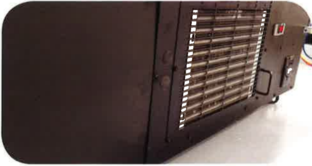
The air intake grill (located at foot traffic level) is prone to suck in ground dirt, carpet lint and food ingredients along with necessary fresh air.
